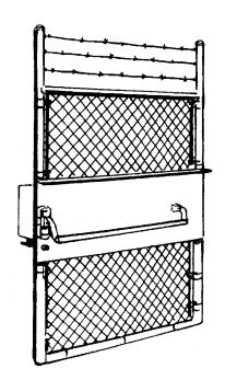
Panic hardware gates can replace your existing standard chain link man gates for faster emergency exits, and can be installed on any size of steel post.
