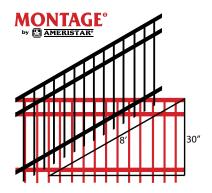
The ATF® (All Terrain Fence) panel design enables the maximum bias for all Montage™ styles.
