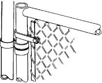
This hinge reduces clearance between frame and gate to approximately 3/8". It is made for square welded gates. The gate itself (one side) becomes part of the hinge assembly, and takes the place of the regular frame hinge.
